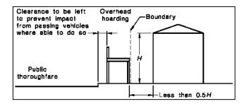
The Principal Contractor or Owner-builder must ensure that overhead protective structures are installed and maintained in accordance with the NSW "*Code of Practice - Overhead Protective Structures 1995*". This is code available at <a href="http://www.safework.nsw.gov.au/\_\_data/assets/pdf\_file/0008/52883/Overhead-protective-structures-Code-of-practice.pdf">www.safework.nsw.gov.au/\_\_data/assets/pdf\_file/0008/52883/Overhead-protective-structures-Code-of-practice.pdf</a>
